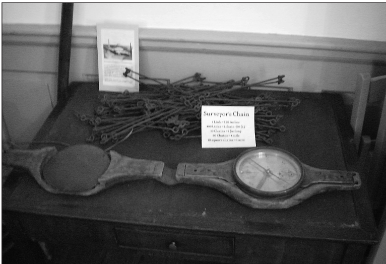
Figure 4. This surveyor's compass (circumferentor) and chain are held on permanent display at Smithfield Plantation in Blacksburg. Both the circumferentor and the 66-link chain seen here have no historical association with William Preston. However, they are similar to those that would have been used by him and his deputies.
